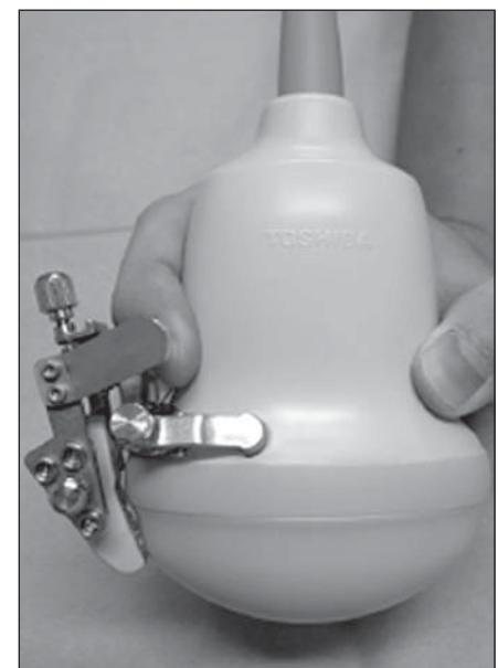
Fig. 2 —Appearance of mechanical volumetric data acquisition (4D) probe with puncture device used in this study. Image used with permission of Toshiba.
