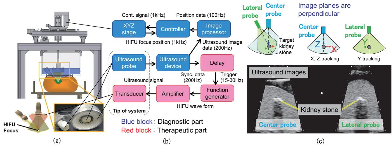
**Fig. 5.** System configuration of an NIUTS. (a) Overview of system configuration. (b) Block diagram of system. (c) Probe configuration and acquired ultrasound images for kidney stone model in ultrasound kidney phantom model.
