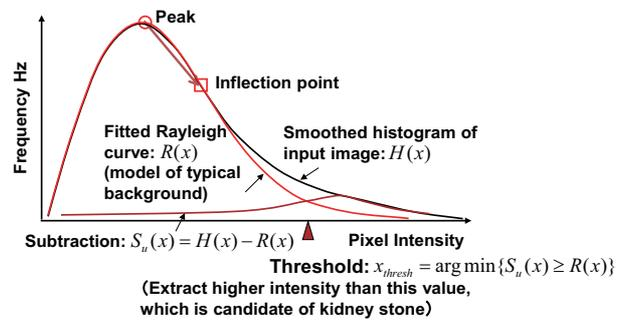
Fig. 7. Automatic thresholding of intensity to extract model kidney stone.
