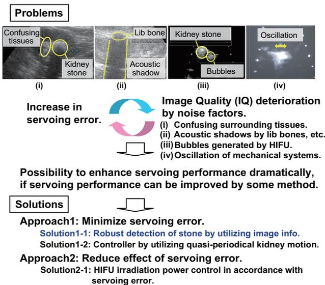
Fig. 6. Problems and solutions with visual motion tracking using ultrasound images.
