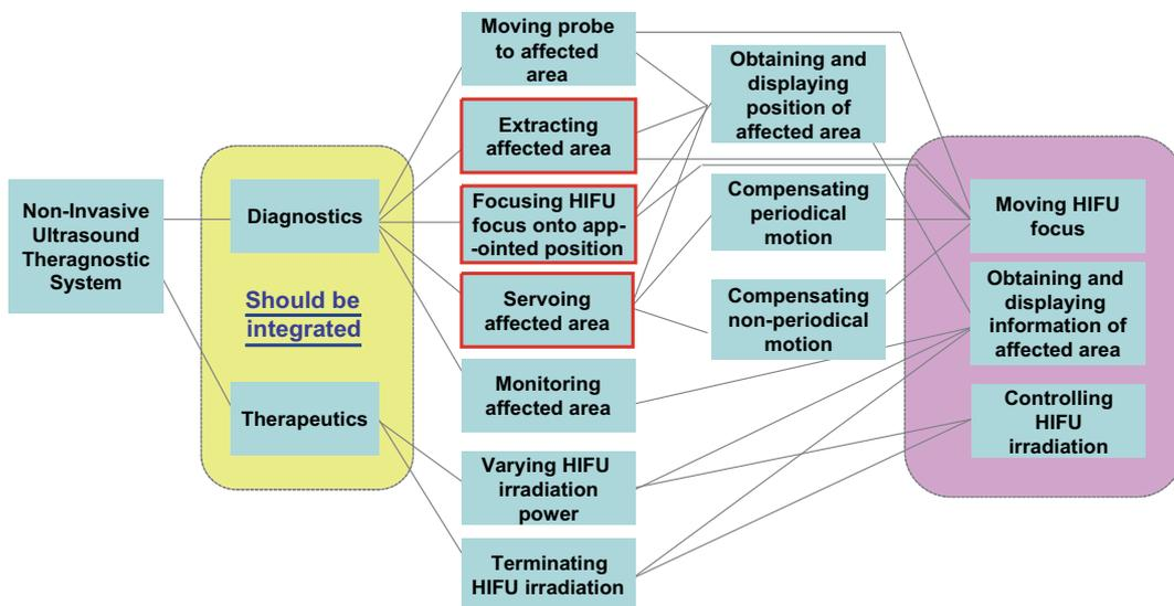
Fig. 4. Required structuring functions for an NIUTS.
